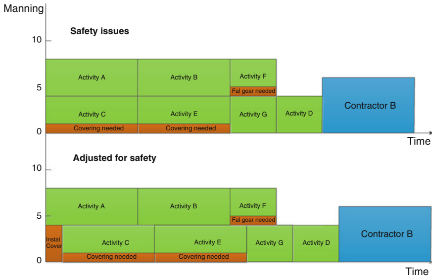
Fig. 11 Example; incorporating safety. Contractor A (marked with green ) is securing a safe working environment by noting and incorporating relevant safety precautions into the schedule. The notes serve as a reminder to safety concerns
